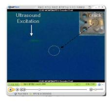
Fig 3. Detection of crack in thick SUS material (14T) with ULT (Lock-in Frequency: 0.2Hz, Ultra sound Power: 1.5kW).
