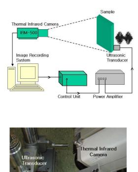
Fig 2. Experimental setup of lock-in thermography with ultrasonic excitation.
