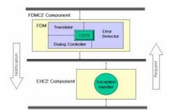
Figure 2. Fault-tolerant COTS software integration architecture
