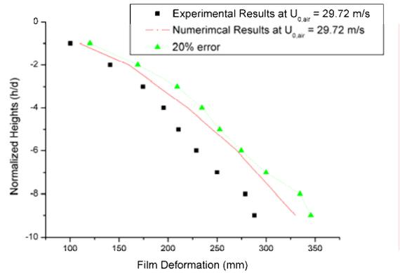
Figure 4. Calculated film deformation at  $u_{0,air} = 29.72$  m/s.
