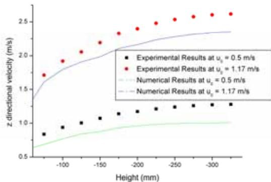
Figure 3. Numerical results of film velocity at the centerline of jet.
