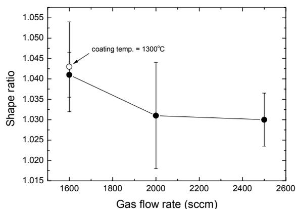
Fig. 3. Variation of shape ratio of the TRISO-coated particles by the coating parameters of the buffer layer.
