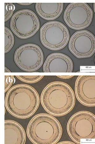
Fig. 1. Microstructures for the cross-sections of the TRISO-coated particles. The gas flow rate for the buffer coating was (a) 1600 and (b) 2500 sccm.
