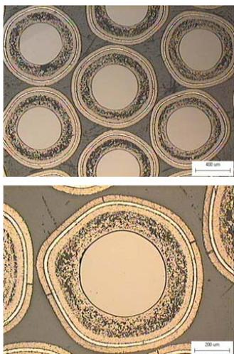
Fig. 2. Microstructures for the cross-sections of the TRISO-coated particles with the buffer layer coated at 1600 sccm and 1300°C.
