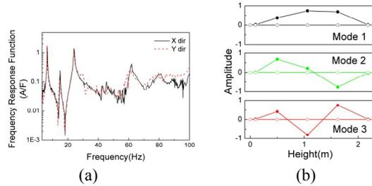
Fig. 2 (a) Frequency response function (A/F) of the test bundle for the two perpendicular vibration directions, (b) mode shapes of the test bundle.
