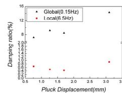
Fig. 5 Damping ratio of the bundle according to pluck displacement.
