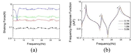
Fig. 3(a) Input shaking force history v.s. swept frequency, (b) Frequency response function (A/F) of the test bundle.
