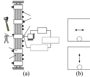
Fig. 1 (a) Vibration test overview, (b) vibration direction and empty region (dotted) within the test bundle's cross section.
