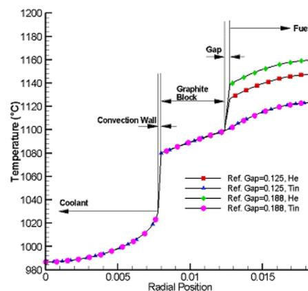
Figure 3. Temperature distributions in the coolant channel.
