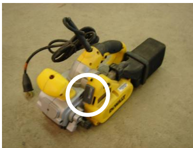
Figure 4. RFID Tag attached on a tool
