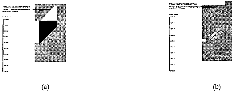
Fig. 2. Density distribution at the (a)beginning and (b)end of uniaxial compression for W-Cu composite powder
