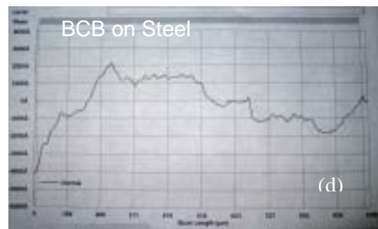
Figure 3. Measures of surface roughness: (a) and (c) are obtained for bare SS substrate, and (b) and (d) are obtained after coating a double-layer of SOG and a single-layer BCB, respectively.
