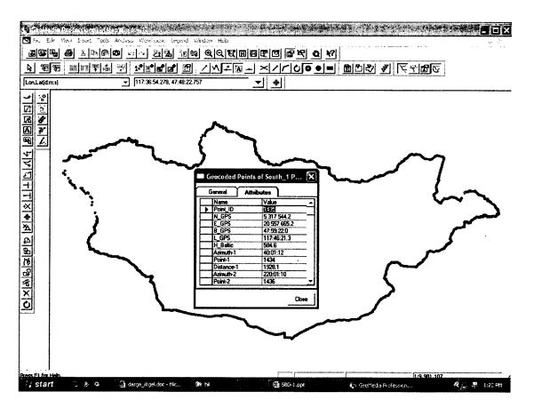
Geodetic point database of Ulaanbaatar city was established by using around 2289 point information of triangulation, polygon meter, gravimeter, level and GPS networks.
