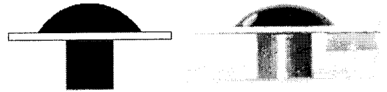
(a) Computed shape (b) Photographed shape Fig. 4 Shapes of the magnetic fluid under the magnetic field and gravitation
