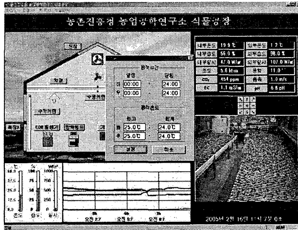
Fig. 2 A view of control program of greenhouse control system.
