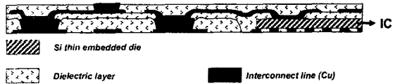
Figure 12: Schematic cross-section of the UTCF foil after removal of the sacrificial substrate.
