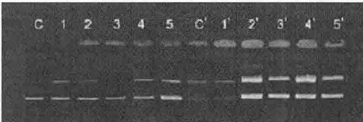
Fig. 2. Agarose-gel electrophoresis of plasmid DNA irradiated with \gamma - radiation. The C-5 is pBR 322 and C'-5' is \phi X174 RF DNA : C,C', control; 1,1', 7.5Gy(37.5ppm of BSH); 2,2' 7.5Gy(75ppm); 3,3', 15Gy(150ppm); 4,4', 30Gy(75ppm); 5,5', 30Gy(150ppm).
