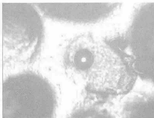
Figure 1. Optical microscopy of a uranium metal particle of 70 \mu\text{m} in diameter on a 1x1 mm carbon tape
