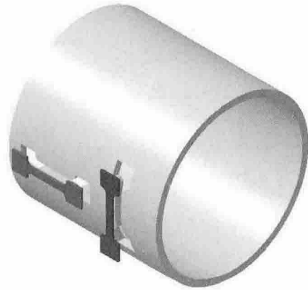
Figure 1. Schematic of uniaxial creep specimen.
