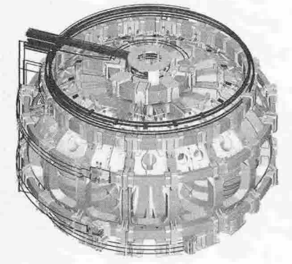
Fig 2. 3D drawing of He line routing in-cryostat.
