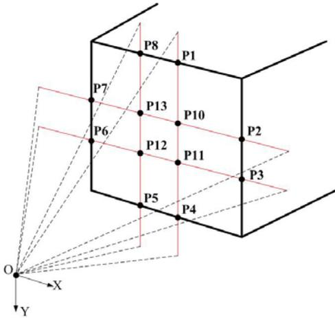
Fig. 6 Coordinate of the Line-laser Image and The Billet (Coordinate of 12 points)
