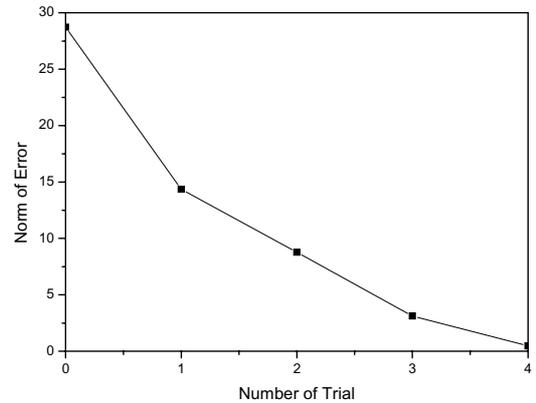
(e) The position error between two centers as the location tracing algorithm is running
