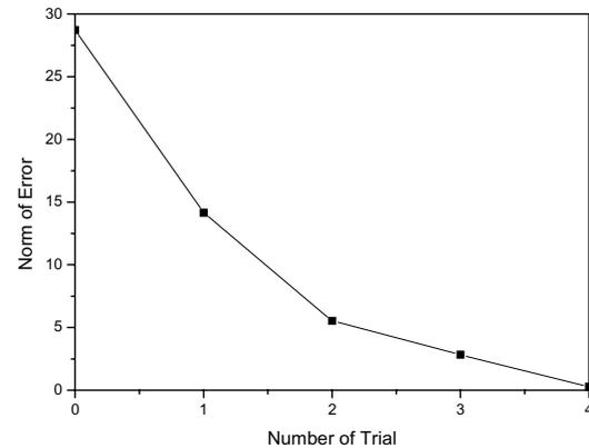
(e) The position error between two centers as the location tracing algorithm is running
