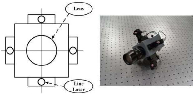
Fig. 2 Laser Position Detecting Sensor System
