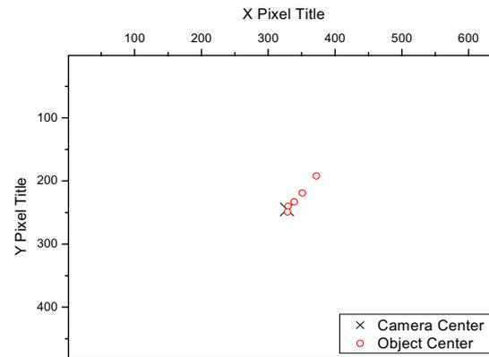
(d) The positions of camera center and billet center as the location tracing algorithm is running
