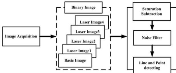
Fig. 4 Schematic Diagram of Pre-Processing
