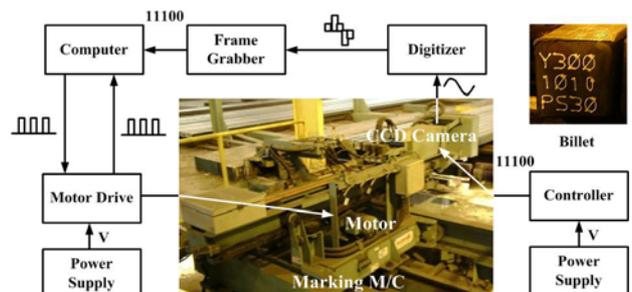
Fig. 1 Billet Automatic Marking System
