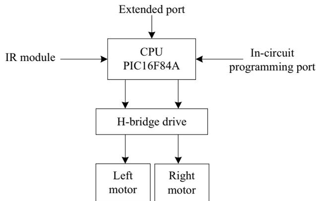
Fig. 4 Structure of control circuit.
