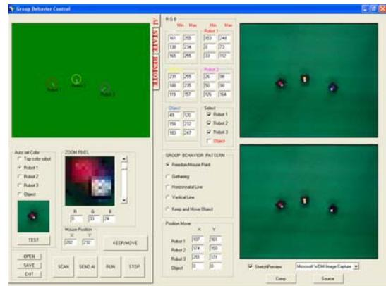
Fig. 8 GUI for micro robotic system.
