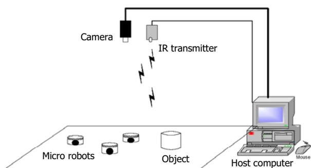
Fig. 1 System configuration.
