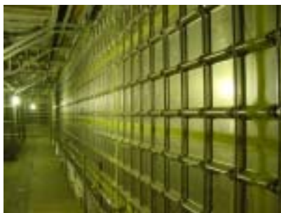
Fig. 1 The LNGC tank which consists of many plates
