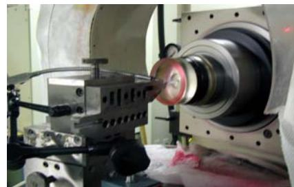
Fig. 2 Lens Polishing / Lapping in DTM using Air Spindle (X, Z axis)
