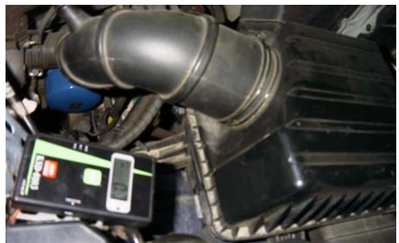
Fig 13. Electrostatic measuring at air filter
