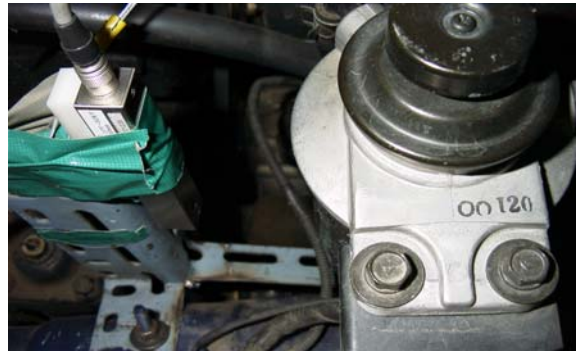
Fig 11. Electrostatic measuring at fuel filter
