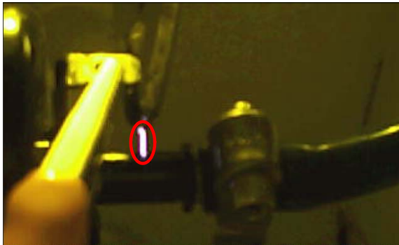
Fig 9. Electrostatic discharge at -30°C
