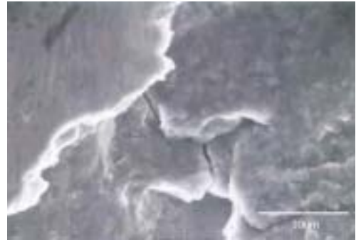
Fig. 6 Observation of worn surface in I-600
