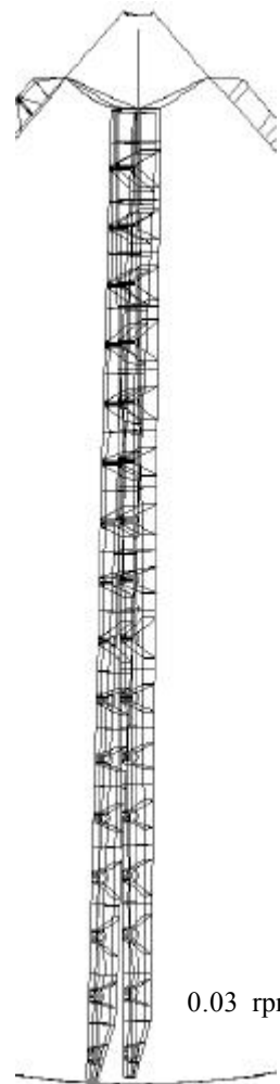
Fig. 5 Schematic of the rotating sludge header
