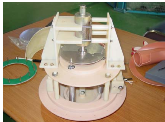
Fig. 4 Valve for a Pressurization System
