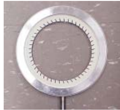
Fig. 2 Reactor ring with thermal barrier coating
