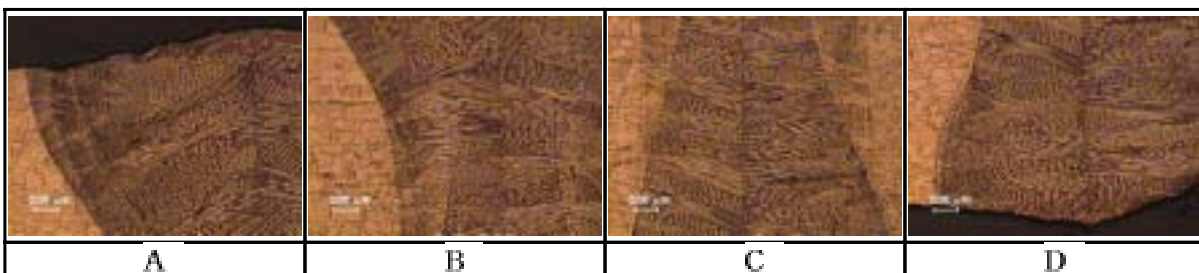
Fig. 8 Photographs showing laser butt welding( P=1.6kW , v=1.0m/min , z=0.5mm )
