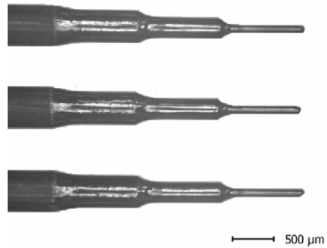
Fig. 7 Fabrication results of three microelectrodes
