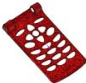
Fig.8 FE (ANSYS) models from the Scanned Data Without CAD modeling
