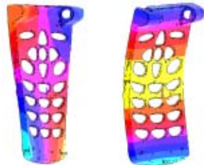
(a) Twisting Mode (b) Bending Mode Fig.9 1 st and 2 nd modes
