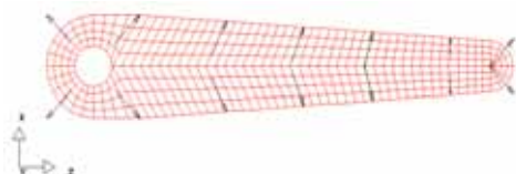
Fig. 9 Design variables for the shape optimization of the connecting rod
