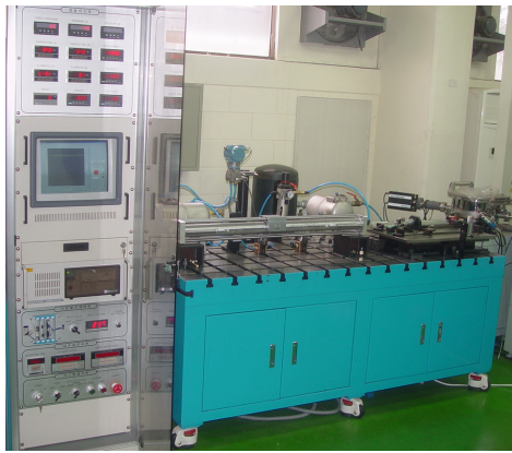
Fig. 7 Measurement Apparatus of Friction Force
