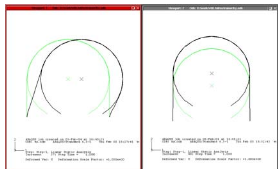
Fig.2 Deformation analysis of the U Strainer
