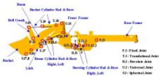
Fig. 1 Dynamic model of a wheel loader
