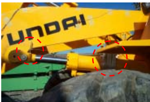
Fig. 6 Measurement for boom cylinder displacement
