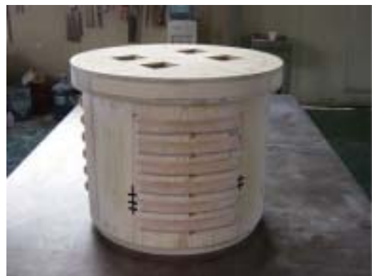
(a) Mold for an inner part of a manhole
