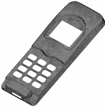
b) Constructed shell mesh on midsurfaces with 25789 triangular elements
