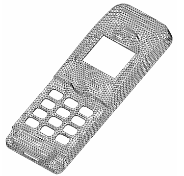
a) Triangulated surface model (13958 input triangular elements)
