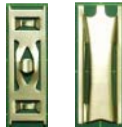
Fig. 5 Test Specimen of KAERI Designed Springs(left: Opt. H; right: Doublet).
