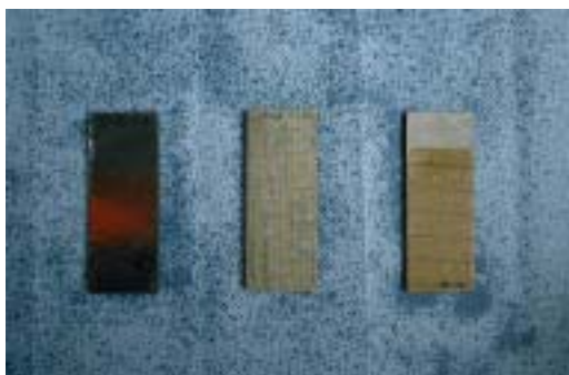
Photo. 2 Insulation specimens of stator winding
