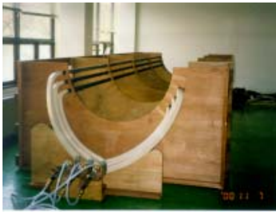
Photo. 4 Test equipment of vibration and wet absorption for winding
