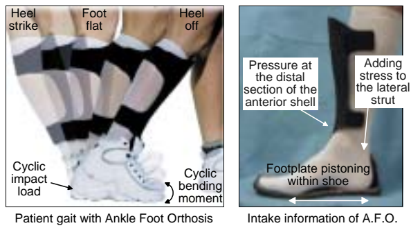
Fig. 1 Schematic view of patient gait with Ankle Foot Orthosis (A.F.O.) and A.F.O. information
