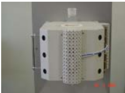
Fig. 1 Furnace for MWCNT purification process.
