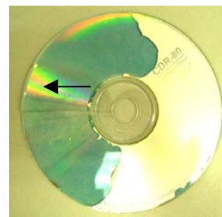
Fig. 3 Failed specimen after 10,500 R.P.M testing
