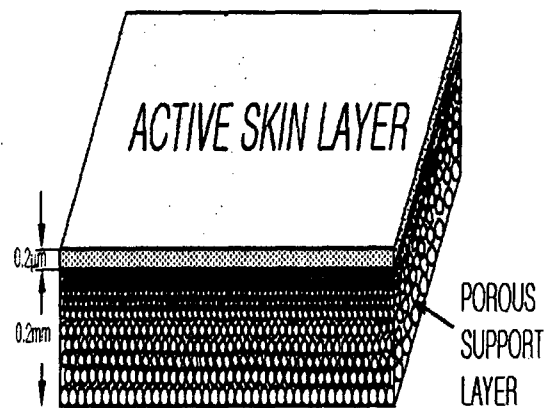
[Fig. 2] Asymmetric structure of traditional RO Membrane
