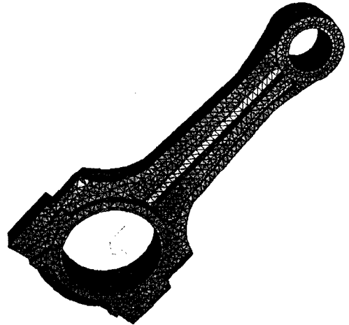
Fig.5 A meshed connecting rod model in ABAQUS
