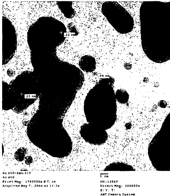
Fig. 3. TEM Image of gold particle(standard sample, 120kV HR mode)
