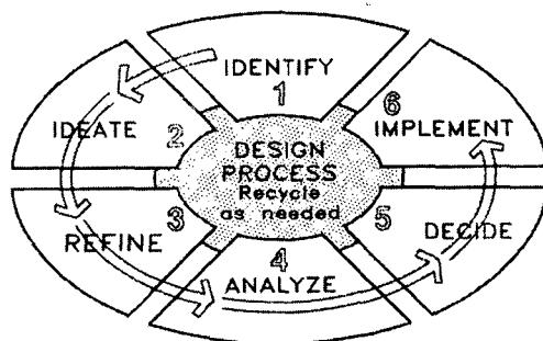
Fig. 1 Six Steps of Design Process
