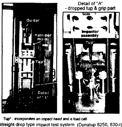
Fig. 1 Impact test machine (weight drop type, Dynatup 8250, 830-I)
