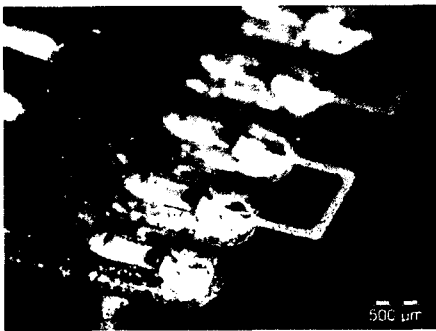
Figure 15: Wetting characteristic of Heraeus Seal V2 on QFP leads, Pitch 0,5 mm
