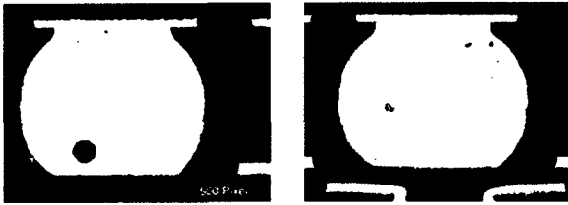
Figure 5: Microsection SACIn- / SACInNd-Ball Interconnection
