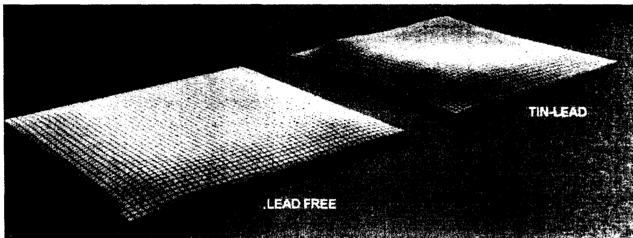
Figure 11- Greater uniformity of coating thickness with Ni-modified Sn-Cu eutectic HASL
