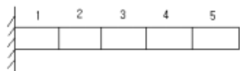
Fig.1 Cantilever beam composed of five elements
