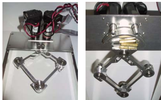
Fig. 9 Front and rear view of five bar mechanism to feedback 2 DOF translational force
