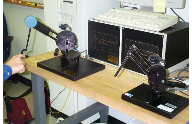
Fig. 7. Phantom haptic devices configured for teleoperation.
